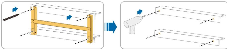
**step 3** Secure the mounting-bracket with bolts.
