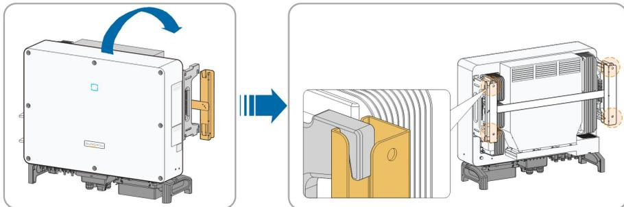
**step 8** Fix the inverter with screws.
