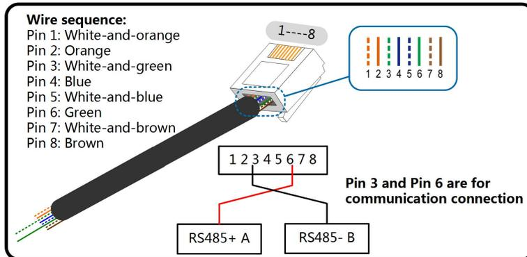
**step 4** Insert the RJ45 connector to the RJ45 jack.
