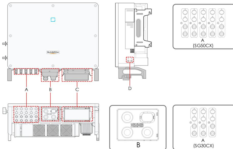
figure 5-1 Wiring terminals
