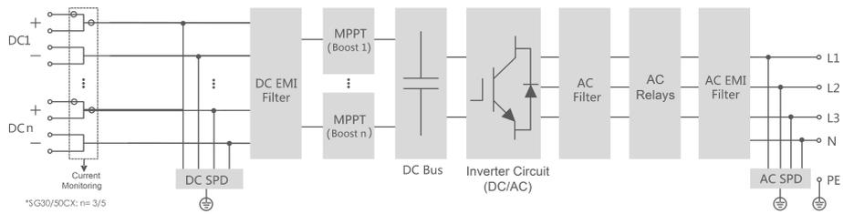
figure 2-3 Circuit diagram
