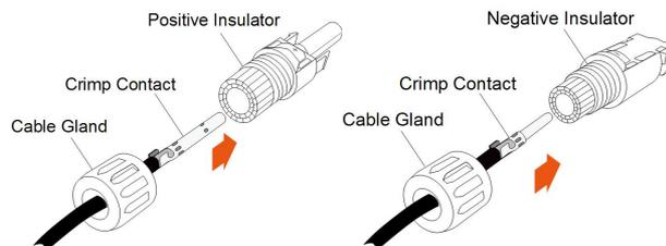
**step 4** Check for polarity correctness.
