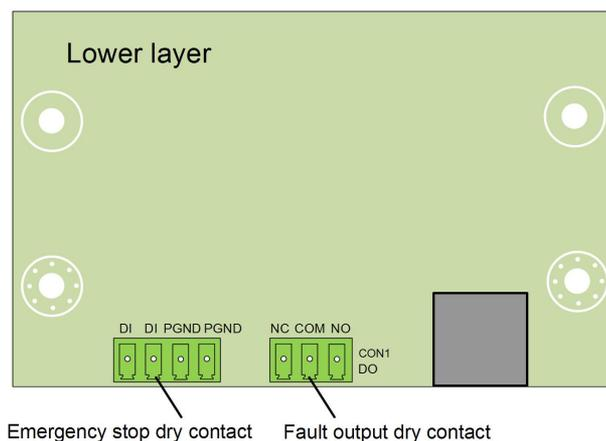
**DO terminal (fault output dry contact):** the relay can be set to fault alarm output, and user can configure it to be a normal open contact (COM&NO) or a normal close contact (COM&NC).
