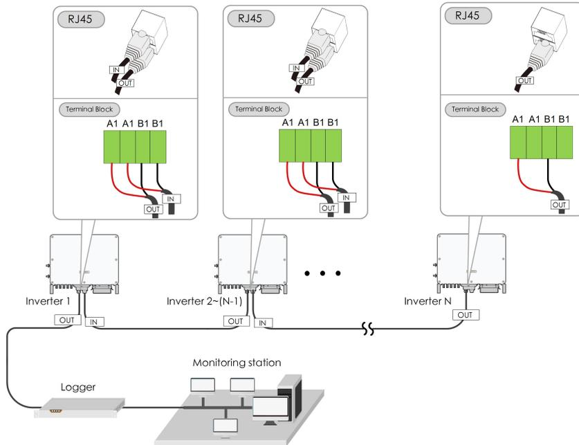
When more than 15 inverters are connected on the same daisy chain, the inverters on two ends of the chain should be equipped with terminal resistors of  $120\Omega$  to ensure communication quality by configuring the dip switch (SW1), and the shielding layer of the communication cable should be single-point grounded.
