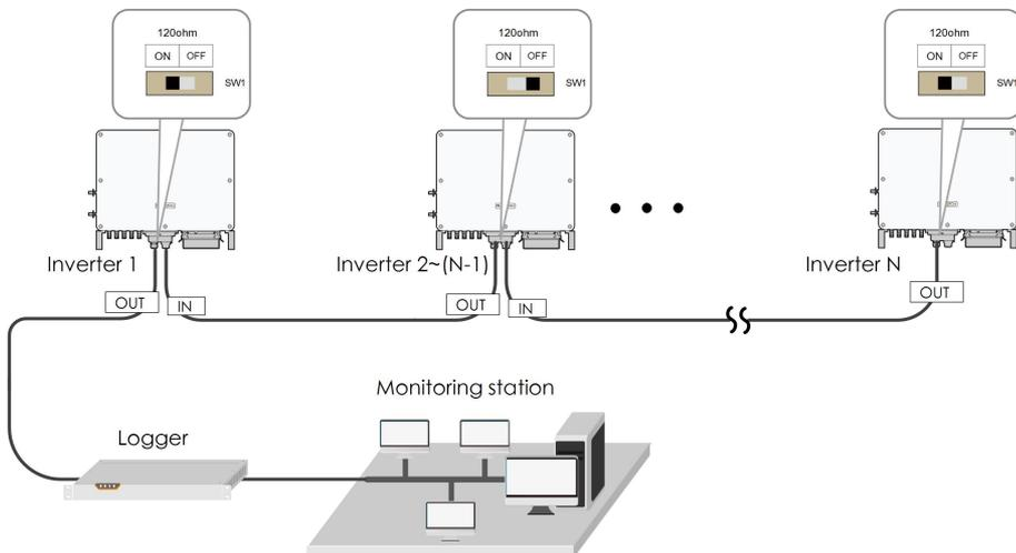
figure 5-4 Configuration of dip switch ( $N \geq 15$ )
