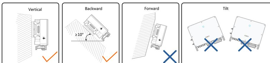
In case the installation site is a level surface, mount the inverter to the horizontal-mounting bracket to meet the mounting angle requirements, as shown in the figure below.
