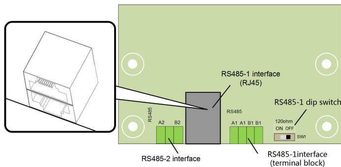
All the three interfaces can be connected to a data acquisition device (Logger), to achieve data exchange with PC or other monitoring devices.
