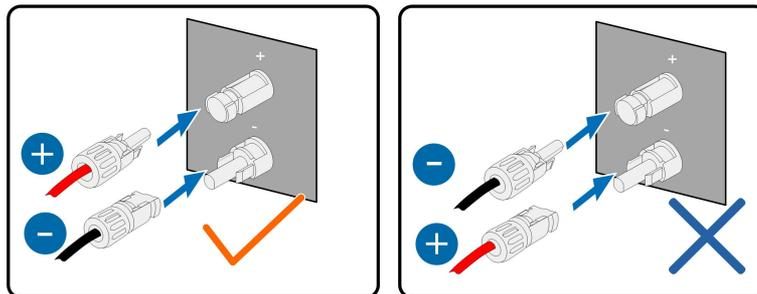
Arc or contactor over temperature may occur if the PV connectors are not firmly in place, and SUNGROW shall not be held liable for any damage caused.
