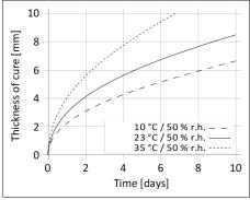
Diagram 1: Curing speed Sikaflex®-554
