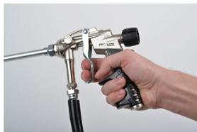
7. Adjust the spray pattern by turning the black valve on the spray-gun anti-clockwise until a spray pattern width of ~300 mm in width is achieved.
