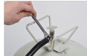
3. Attach the other end of the rubber hose to the spray-gun (using the large nut). Tighten with a spanner.
