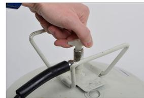
2. Unscrew the hose from the canister valve.
