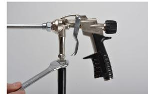
4. Using the locking-nut provided, attach the spray-tip to the end of the spray-gun.
