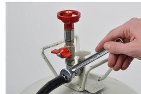
4. Check the tap on the assembly is off before applying the Sika Spray Cleaner. Screw the Sika® Spray Cleaner canister into the top of the assembly and open the red valve.
