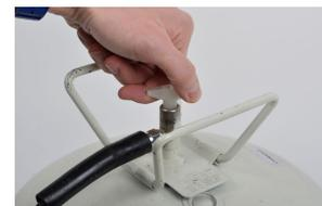
6. Pull the trigger on the spray-gun to apply adhesive.
