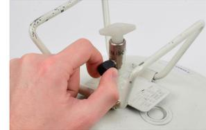
2. Attach the rubber hose to the canister valve (using the small nut) and attach the other end of the braided-hose to the spray-gun (using the large nut). Tighten with a spanner.
