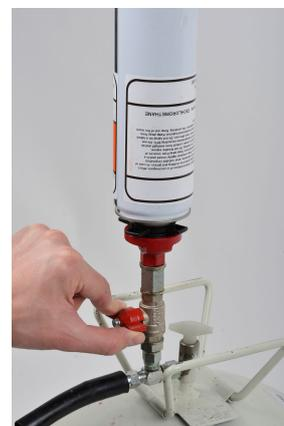
5. Aim the spray-gun into a waste container, apply pressure to the trigger on the gun to push Sika® Spray Cleaner through the hose and gun until the adhesive starts to dispense. Keep pressure on the trigger until the hose and gun are thoroughly cleaned.
