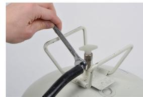
3. Attach the assembly to the valve. Ensure the assembly remains upright whilst the nut is tightened. Attach the hose to the assembly. Ensure the assembly remains upright whilst the hose nut is tightened.
