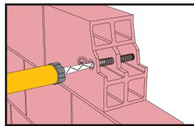
Inject the adhesive into the perforated sleeve, starting from the bottom, while slowly drawing back the static mixer. In any case avoid entrapping air.
