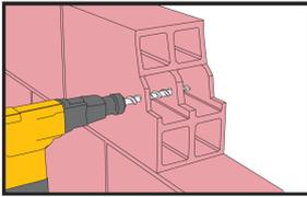
Drilling of hole with an electric drill to the diameter and depth required. Drill hole diameter must be in accordance with anchor and perforated sleeve size. Note: with hollow material do not use rotary hammer drills.
