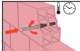
Insert the anchor with a rotary motion into the filled perforated sleeve. Use the adequate steel rod size. Important: the anchor must be placed within the open time.
