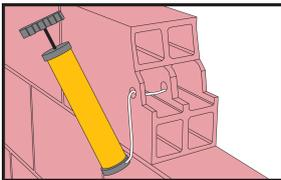
The drill hole must be cleaned after each cleaning step with a blow pump or by compressed air, starting from the bottom of the hole (pump at least 1x). Important: use oil-free compressors.
