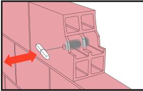
The drill hole must be thoroughly cleaned with a round brush (brush at least 1x). The diameter of the brush must be larger than the diameter of the drill hole.
