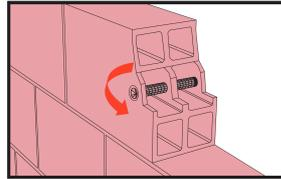
Close the cap from the perforated sleeve to avoid some escape of the resin during entering the steel rod.
