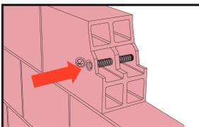
Insert perforated sleeve completely into the drill hole.
