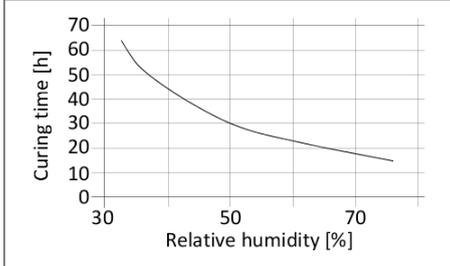
Diagram 1: Curing time for 500 µm film
