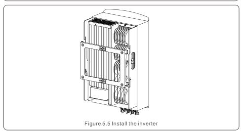
4. Lift the inverter and hang it on the backet, and fixing both sides of inverter with locking screws (accessories).
