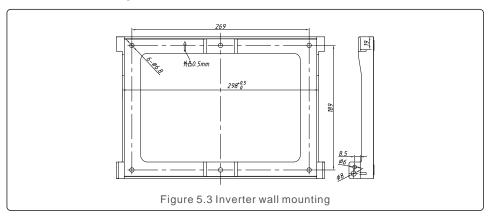
Refer to figure 5.4 and figure 5.5. Inverter shall be mounted vertically.
