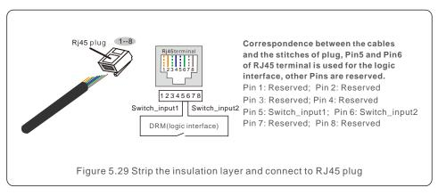
3. Connect RJ45 to DRM (logic interface).
