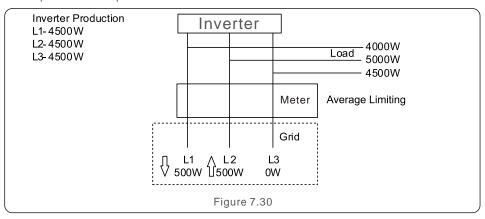
Mode "02", As shown in the figure 7.32 the per phase limiting mode, the inverter only generate the power that equals to one of three-phase load power that is the lowest load power of a certain phase.
