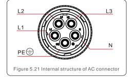
The steps of AC gird terminal connector for install as follows:
