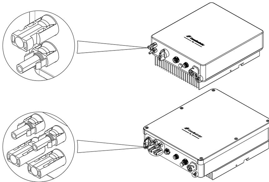
FIG. 7-8 DC Input Connectors
