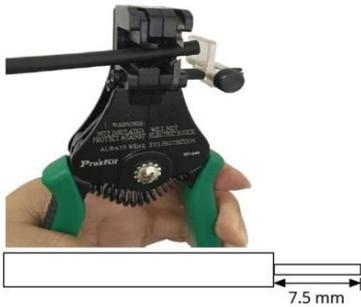
FIG. 7-10 Strip the Cable Insulating Layer
