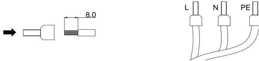
FIG. 7-4 Crimp the Three-core's Ferrule
