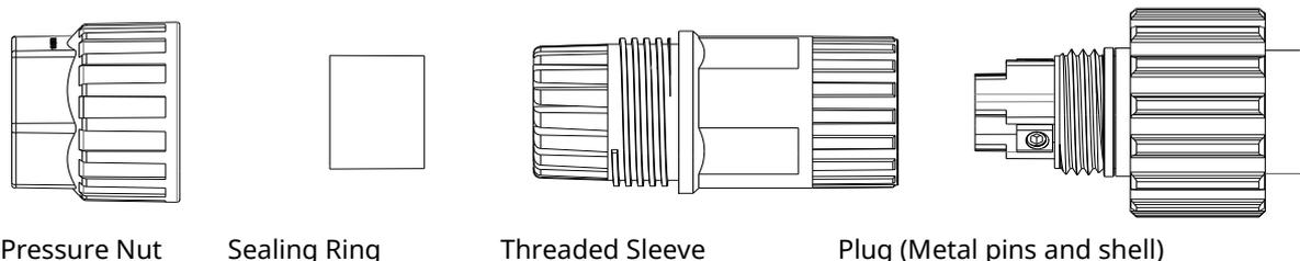
FIG. 7-2 Components of Connector
