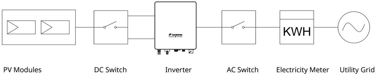
FIG. 3-1 PV Power System Diagram
