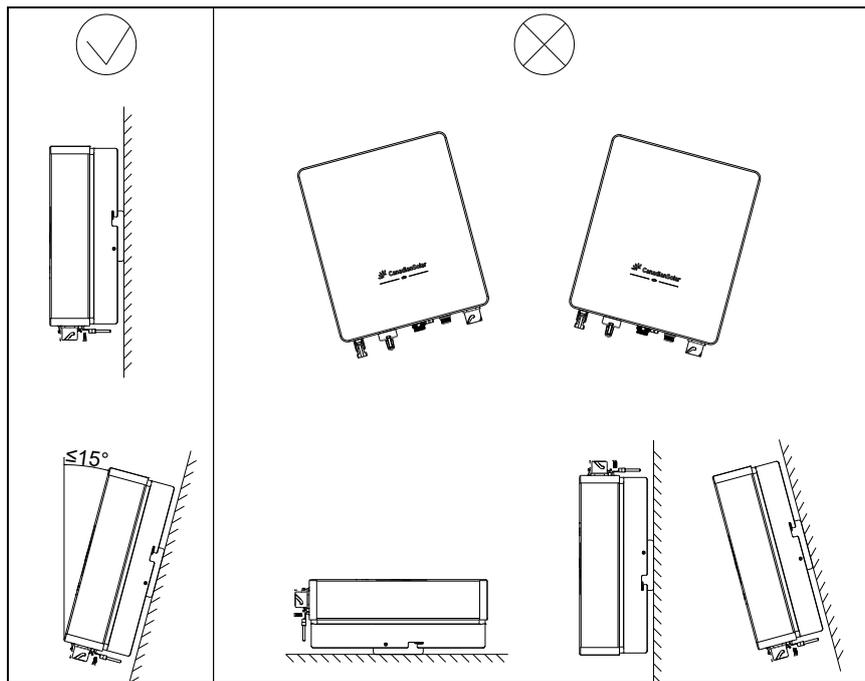
FIG.6-5 Installation Angle Requirements
