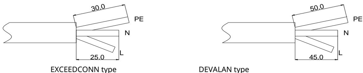
FIG. 7-3 Adjust the Cable Length
