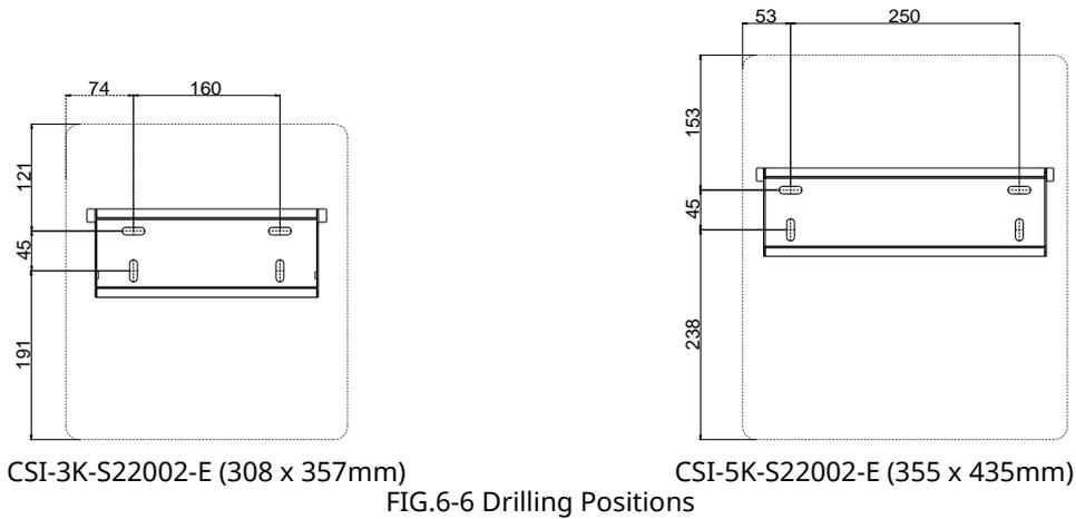
2) Drill expansion anchors into the corresponding four holes, and then secure the bracket by using screws, as per FIG. 6-7 & FIG. 6-8.
