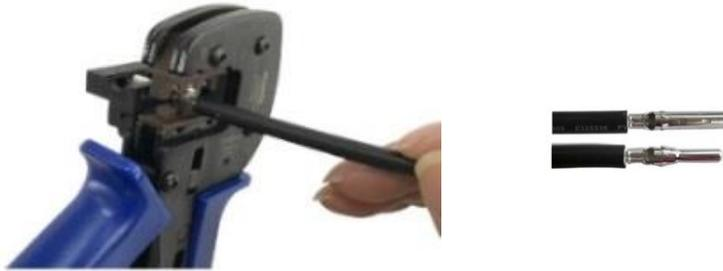
FIG. 7-11 Crimp the Contact
