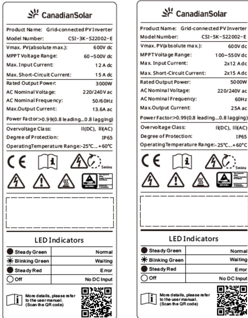
FIG.3-3 Inverter Nameplate (for reference)
