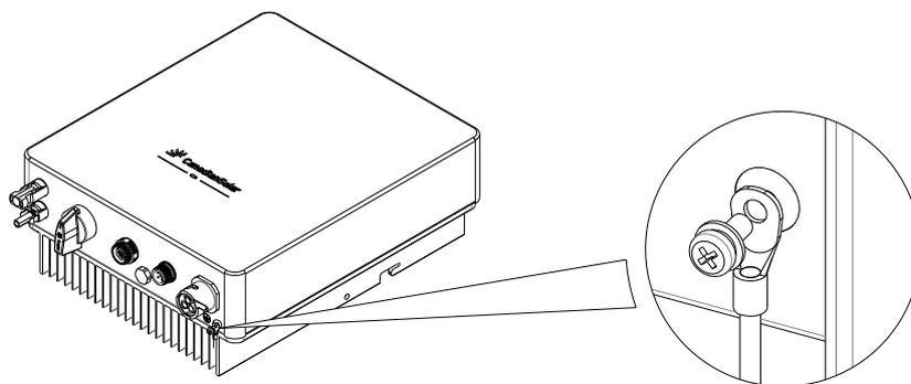
FIG. 7-1 External Grounding Point Position
