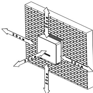
FIG.6-3 Installation Clearance Requirement
