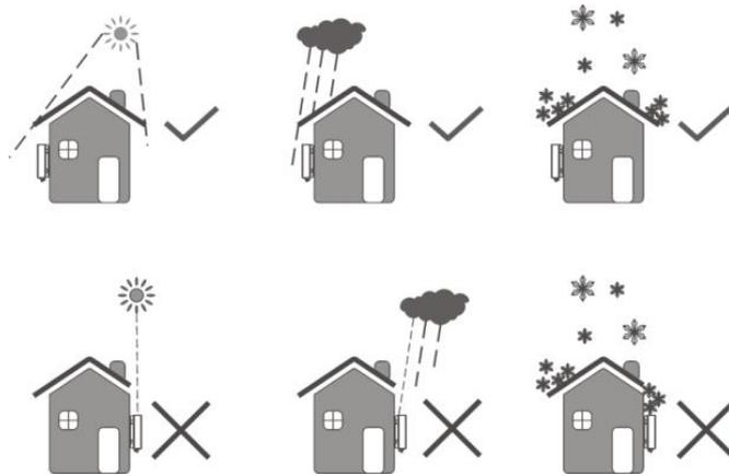
FIG.6-1 Inverter Installation Positions
