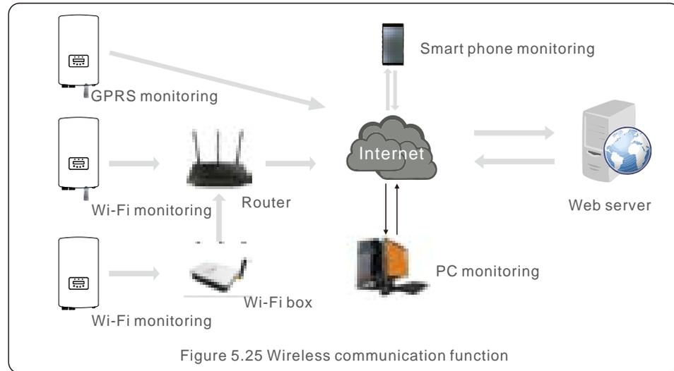
Figure 5.25 Wireless communication function
