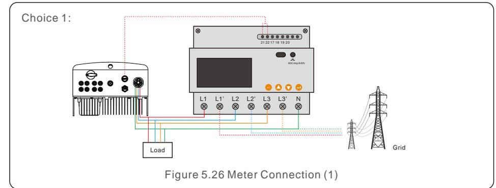
Figure 5.26 Meter Connection (1)
