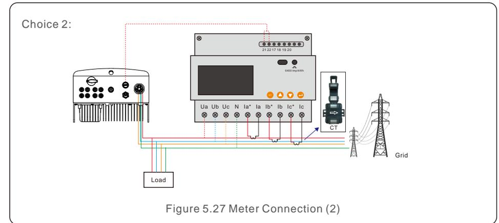
Figure 5.27 Meter Connection (2)
