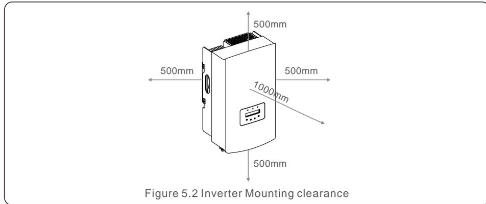
Figure 5.2 Inverter Mounting clearance
