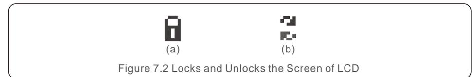
Figure 7.2 Locks and Unlocks the Screen of LCD
