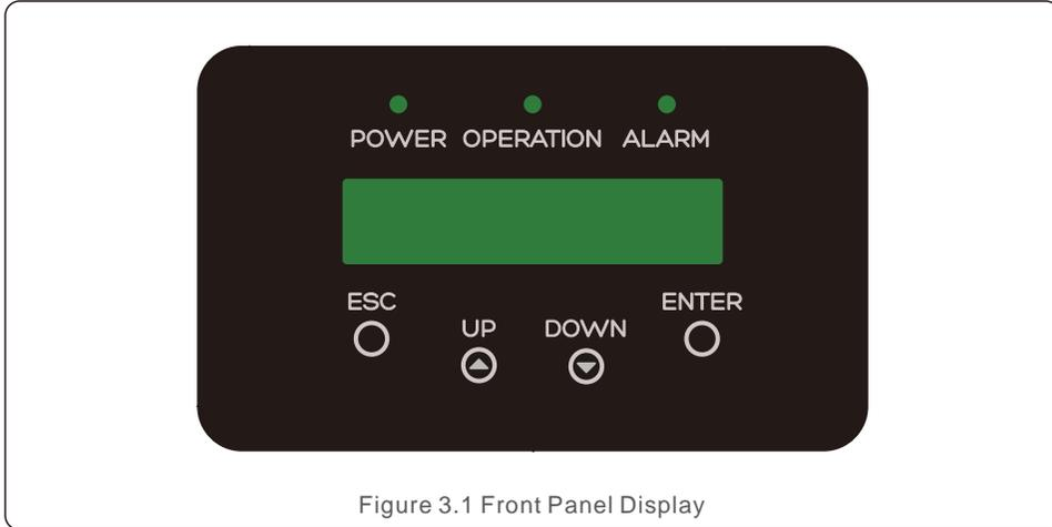
Figure 3.1 Front Panel Display
