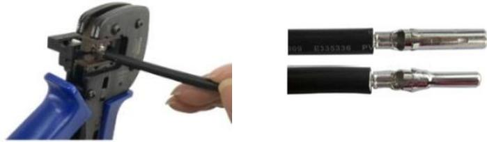
FIG. 7-12 Crimp the Contact
