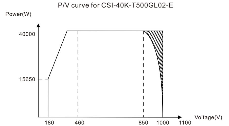
▲ Figure 10.6 CSI-40K-T500GL02-E Inverter output power by input voltage
