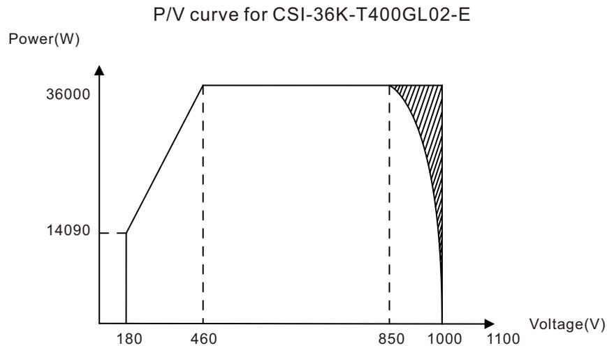
▲ Figure 10.4 CSI-36K-T400GL02-E Inverter output power by input voltage
