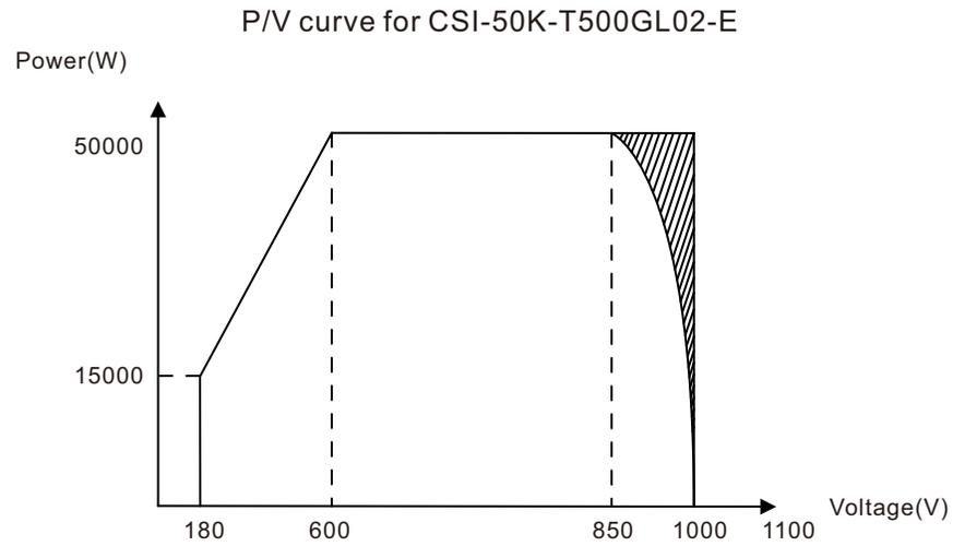
▲ Figure 10.7 CSI-50K-T500GL02-E Inverter output power by input voltage
