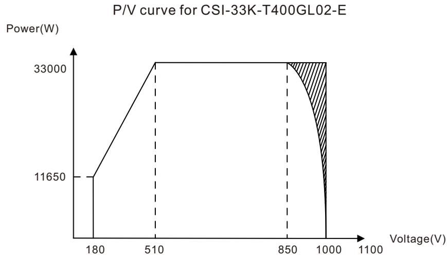
▲ Figure 10.3 CSI-33K-T400GL02-E Inverter output power by input voltage
