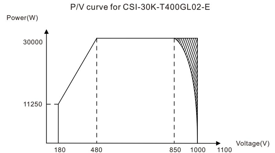
▲ Figure 10.2 CSI-30K-T400GL02-E Inverter output power by input voltage
