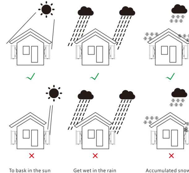
Figure 5.1 Recommended Installation locations
