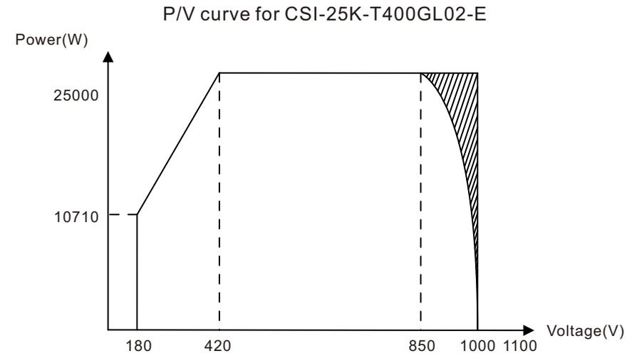
▲ Figure 10.1 CSI-25K-T400GL02-E Inverter output power by input voltage
