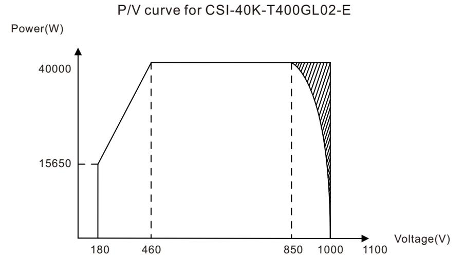
▲ Figure 10.5 CSI-40K-T400GL02-E Inverter output power by input voltage
