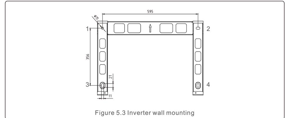
Figure 5.3 Inverter wall mounting
