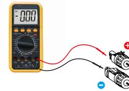
Figure 5.21 Multimeter measurement
