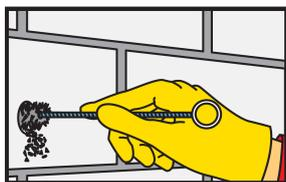
5. The drill hole must be thoroughly cleaned again as per Stage 3.
