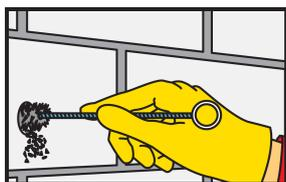
3. The drill hole must be thoroughly cleaned with the special steel brush (brush at least twice). The diameter of the brush must be larger than the diameter of the drill hole.
