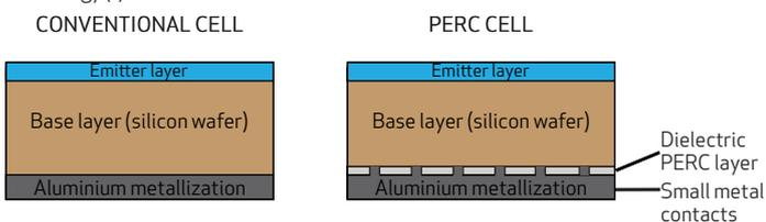
Although the passivation layer cannot be seen in the cells and makes no difference to the visual appearance of the panel, it boosts overall module power in two distinct ways.
