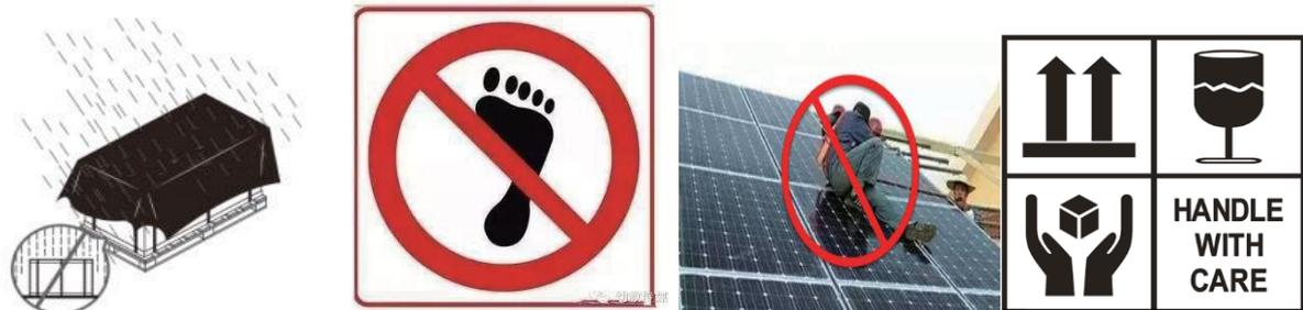
Figure 4 operation safety diagram of module
