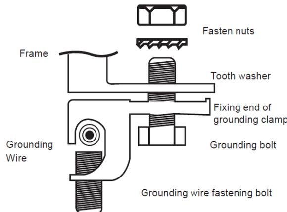
Figure 15 Bolt Grounding Method
