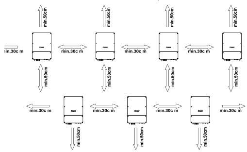
FIG.6-4 Staggered Installation Mode (Recommended)
