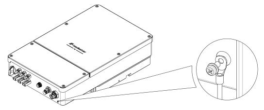
FIG. 7-1 External Grounding Point Position
