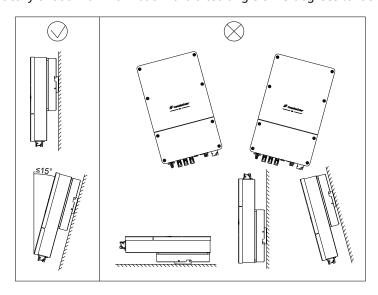
FIG.6-5 Installation Angle Requirements
