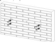
FIG.6-7 Install Expansion Anchors
