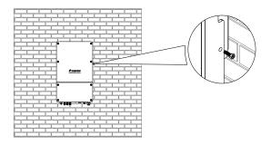
FIG. 6-10 Fix Both Sides of Inverter
