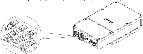
FIG. 7-9 DC Input Connectors
