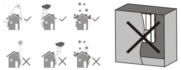
FIG.6-1 Inverter Installation Positions
