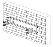
FIG.6-8 Fix Wall-mounting Bracket
