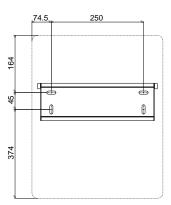
FIG.6-6 Drilling Positions (W x H, 399 x 583mm)
