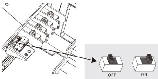
If multiple inverters adopt daisy chain communication configuration, the configuration method of 485 bus matching resistance is suggested as follows:
