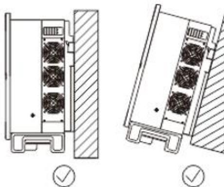
12. Never install the inverter horizontally, or with a forward tilt or with a backward tilt or even with upside down. The horizontal installation can result in damage to the inverter.
