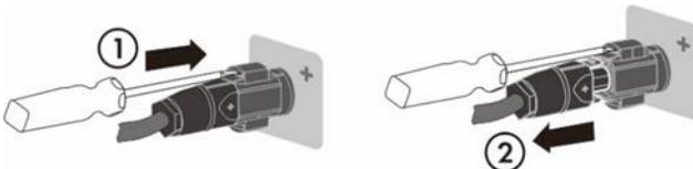
5. Release and disconnect the AC connector. Unscrew the screws of the AC terminals, and then pull out the AC connector.
