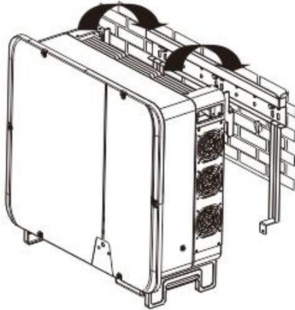
5. Check both sides of the outer fin of the inverter to ensure that it is securely in place.
