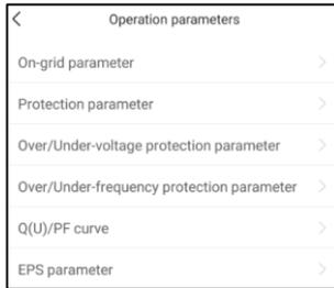
For convenient protection parameter setting, the protection parameters are preset for certain countries. After country setting, select the protection stage as single or multiple and then set the corresponding protection parameter.
