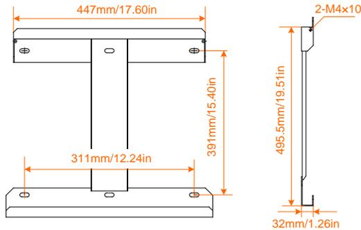
**Fig. 5-1** Dimensions of the bracket (figures in inch)
