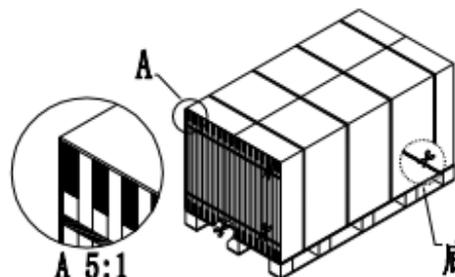
4.3.7 When unpacking on a level surface, take out the module from one side of package to the other, and then carry it with two persons (Please refer to 3.1.8) When unpacking on a sloping surface, please protect the modules from tipping over or sliding. As shown below.
