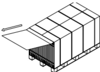
4.3.6 Cut the two horizontal packing belts in the carton and cut the two packing belts near the bottom of the tray, and remove the packing belts.
