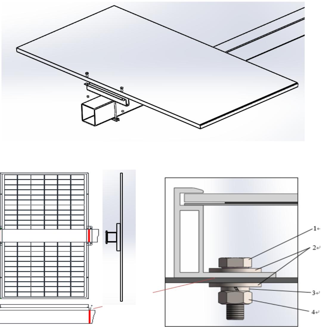
**Fig 5. PV module installed with Single-axis Tracing System**
