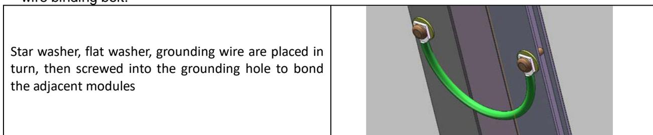
Trina recommends using the following methods to ground installation properly under UL investigation.
