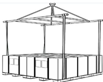
3.2.2 If the condition permits, use a fork lift to remove the module pallets from the truck
