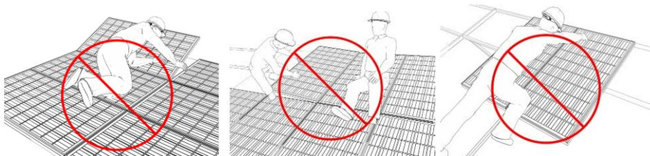
Do NOT damage or scratch the front or backside surfaces of the module.
