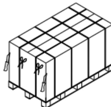
4.3.5 Cut the tape at shorter edge and hold it up by 90° from the bottom; and pull out the cardboard to expose the modules.
