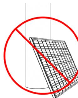
4.3.9 If all the modules are NOT removed after unpacking and some of them are left in the package, the remaining modules shall be laid flat and repackaged to prevent from falling down. Must be placed by horizontal. The stacked number of modules: All frame modules to be stacked NOT more than 16 pieces;
