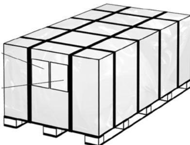
4.3.4 Cut the two packing belts at shorter sides of the tray with blade or scissors, and unpack the side surface of the carton along the vertical direction.
