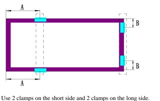
Mounting rails run perpendicular to the long side frame. (fixture length  $\geq$  40mm ,A = (250 - 450) mm,B = (100 - 250) mm
