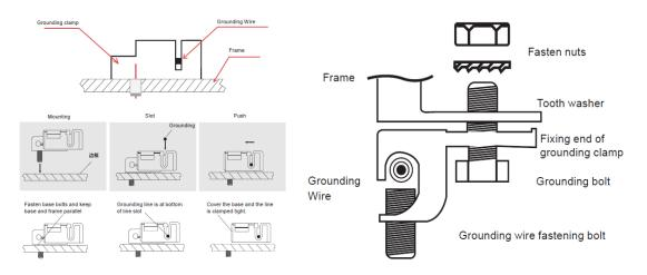
Figure 14 Clamp Grounding Method
