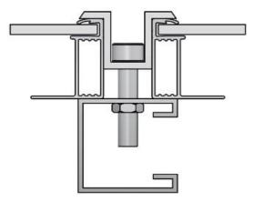
Figure 12 Clamp Installation of Bifacial Module
