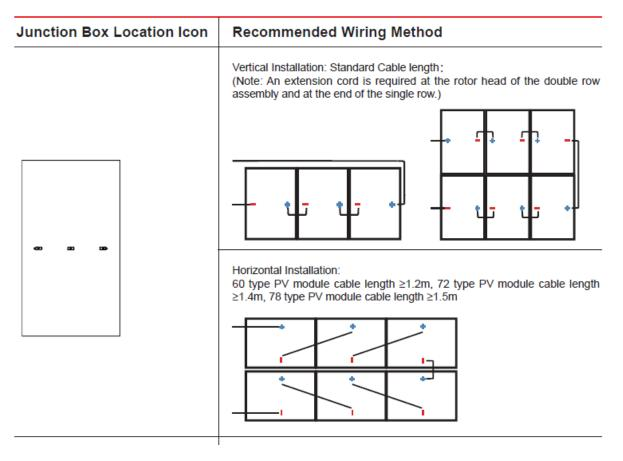
Figure 3 Junction Box Style and Wiring Method
