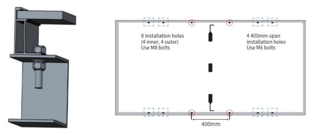
Figure 6 Schematic diagram1 of monofacial module with bolt Installation
