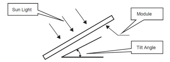
Figure 5 Schematic diagram of component inclination
