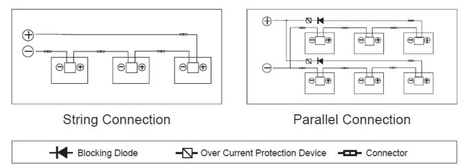
Figure 13 Series Connection and Parallel Connection Circuit Diagram
