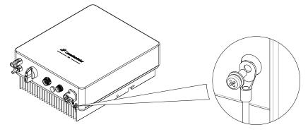
FIG. 7-1 External Grounding Point Position
