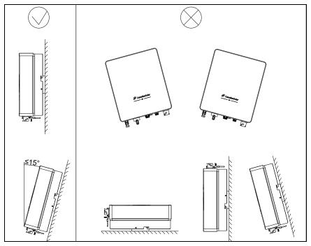
FIG.6-5 Installation Angle Requirements
