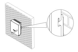
FIG. 6-9 Hang the Inverter on Wall-mounting Bracket
