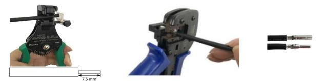
FIG. 7-10 Strip the Cable Insulating Layer
