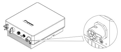
FIG. 7-7 Installing the AC Connector
