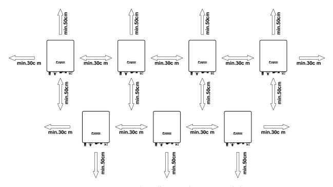
FIG.6-4 Staggered Installation Mode (Recommended)
