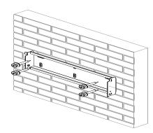
FIG.6-8 Fix Wall-mounting Bracket
