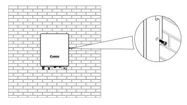
FIG. 6-10 Fix Both Sides of Inverter
