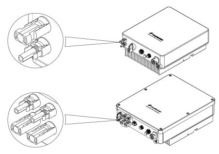
FIG. 7-8 DC Input Connectors
