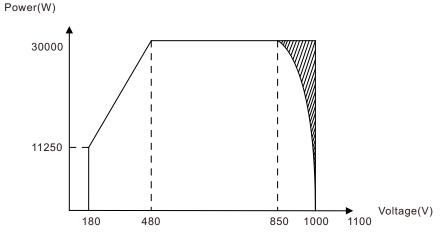
▲ Figure 10.2 CSI-30K-T400GL02-E Inverter output power by input voltage
