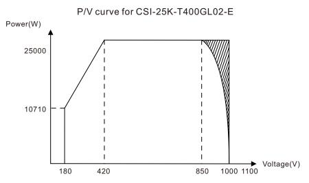
▲ Figure 10.1 CSI-25K-T400GL02-E Inverter output power by input voltage
