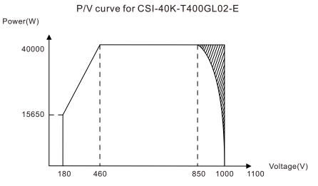
▲ Figure 10.5 CSI-40K-T400GL02-E Inverter output power by input voltage
