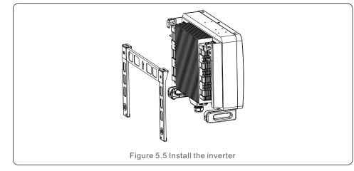
5. Use screws in the packaging to fix the inverter to the mount bracket.
