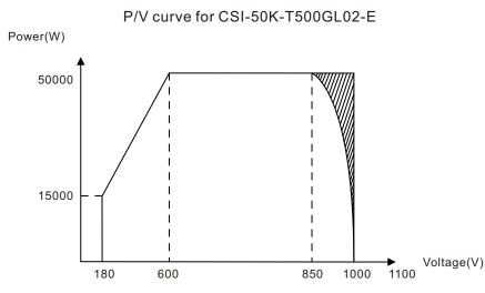
▲ Figure 10.7 CSI-50K-T500GL02-E Inverter output power by input voltage
