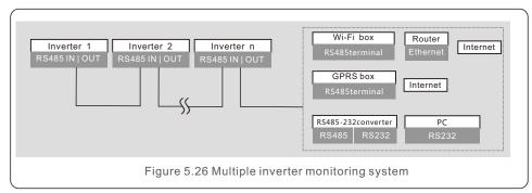
Multiple inverters can be monitored by RS-485 daisy chain configuration. (See figure 5.26).
