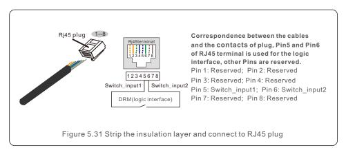
3.Connect RJ45 to DRM (logic interface).
