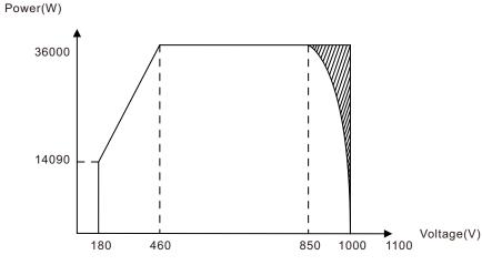
▲ Figure 10.4 CSI-36K-T400GL02-E Inverter output power by input voltage
