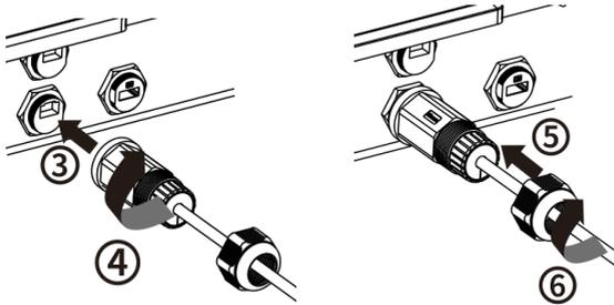
**Disassemble the network cable in reverse order.**
