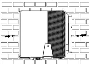
If a second protective conductor is required in installation site, ground the inverter and secure it so that it cannot drop from the housing (see section
