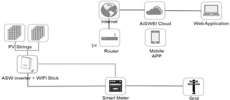
The smart meter should support the MODBUS protocol with a baud rate of 9600 and address set 1. Smart meter as above SDM230-Modbus connecting method and setting baud rate method for modbus please refer to it's user manual.
