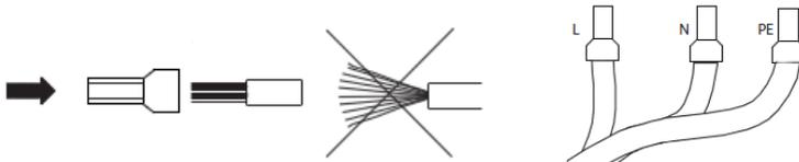
4. Insert the PE, N and L conductor through the AC connector housing and terminate them into the corresponding terminals of the AC connector terminal and make sure insert them to the end in the order as shown, and then tighten the screws with an appropriately sized hex key with a suggested torque of 2.0 Nm.
