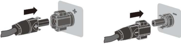
7. Ensure that all DC connectors are securely in place.
