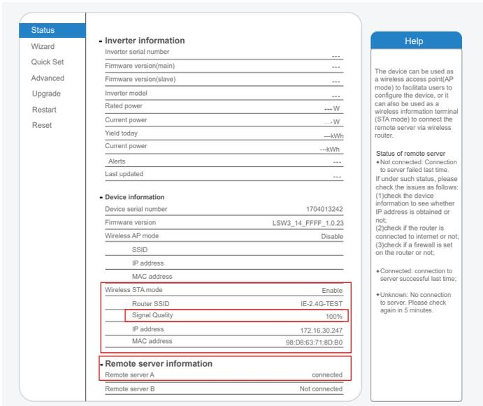
10. If both remote server A and B are "Not connected", please refresh the page or repeat the previous steps. If the "Signal Quality" is lower than 40%, please move your Router closer to the Microinverter.
