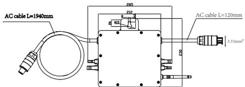
The AC wire on the micro inverter is a TC-ER wire with a wire cross-section area of 3.33mm<sup>2</sup>.
