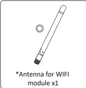
\* This antenna is for microinverter that has built-in wifi module.
