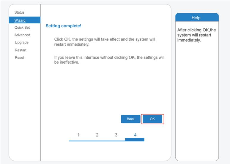
9. Connect to logger AP network again, then log in to 10.10.100.254 by Browser, and check the system info of "Status" page. After the network setting is done, the remote server A or B should be "connected".
