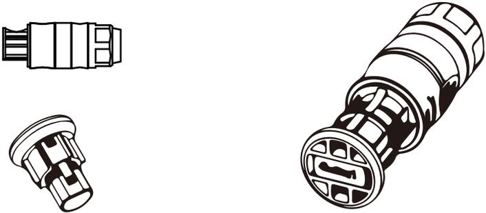
Step 5 - Connect Microinverter to the PV Modules
