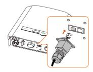
Secure the waterproof lid to the inverter bottom with four screws, then fasten the cable gland.
