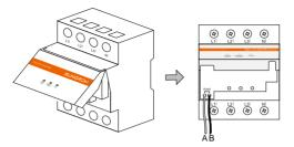
Strip the insulation from the power wires by 10 mm. Then connect the wires to the terminals on the Energy Meter, as shown below. (Cross-section: 10 mm² to 25 mm²)
