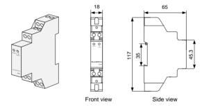
Fig. 2-5 single-phase Meter Dimensions (unit: mm)
