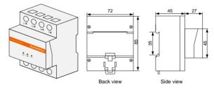
Fig. 2-6 Three-phase Meter Dimensions (unit: mm)
