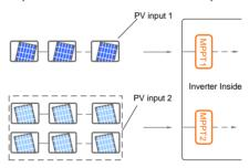
Fig. 5-5 Independent Mode for SG8K3-D
