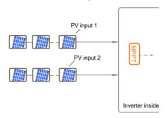
Fig. 5-6 Parallel Mode for -D inverters except SG8K3-D
