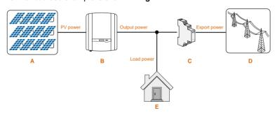
Fig. 2-1 Application in a PV Power System
