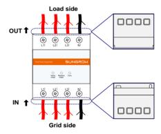
The line conductor L1 supplies power to the Energy Meter. At least the line conductor L1 and the neutral conductor must be connected to the Energy Meter.
