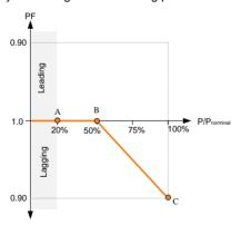
Fig. 2-7 Power Factor Curve
