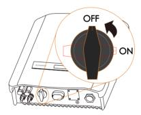
Check the connection cable of the PV string for the correct polarity and that the open-circuit voltage does not exceed the inverter input limit of 600 V, even under the lowest operating temperature. Refer to the module specification supplied by the module manufacturer for detailed information.
