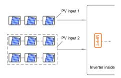
Fig. 5-7 Parallel Mode for SG8K3-D
