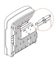
Remove the waterproof lid from RS485 terminal and install the communication module to the inverter. The following figure takes the Wi-Fi module as an example. Refer to the manual delivered with the module for details.
