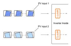
Fig. 5-4 Independent Mode for -D inverters except SG8K3-D
