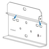
Set the wall mounting bracket aside and drill the marked holes. The depth of the holes should be about 70 mm. Install the wall-mounting bracket.
