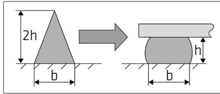
Figure 1: Compressing adhesive bead to final size
