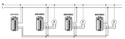
Touch roller shutter modules each connected to a load and wired so they can be commanded via an external command, with the centralised command function.
