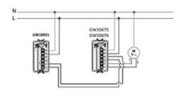
Touch roller shutter module connected to a load and wired so it can be commanded via an external command, with the local command function.
