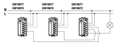
EVO axial one-way switch module connected to a load and wired so it can be commanded via a local command and receive the centralised "OFF only" command
