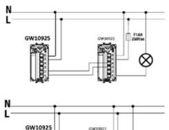
Auxiliary touch control module 2 connected as local or central control of a touch dimmer module
