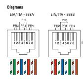
To obtain the EIA/TIA 568A or 568B configuration shown alongside, follow the colour code given on the terminal block (of the products).
