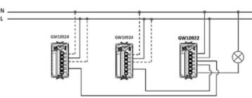
Touch one-way switch module connected to a load and wired so it can be commanded via a local command and receive the centralised "OFF only" command
