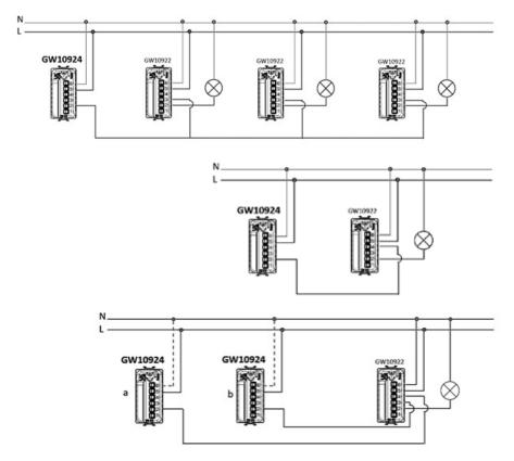
Auxiliary touch control module 1 connected as centralised OFF control to 3 touch switch modules
