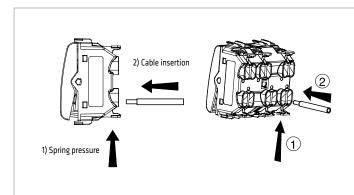
The spring terminals allow you to carry out the wiring in a shorter time, and without using screwdrivers or other tools. To insert the cable, it is necessary to press the orange lever (opening of terminal). Releasing the lever, the terminal closes automatically, firmly blocking the cable.
