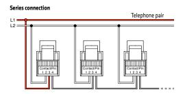
The clamps 3 and 4 are connected by means of the contact inside the telephone, which is closed when the telephone receiver is put down.
