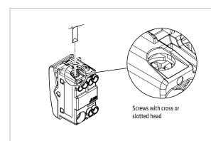
The terminals, located in the rear part of the devices, are manoeuvrable even after coupling the component to the support, and are suitable for both stranded and solid cables. The components are supplied with the screws of the terminals open, to reduce wiring times.
