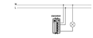
Touch one-way switch module connected to a load
