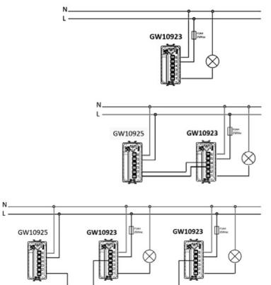
Touch dimmer module connected to a load.
